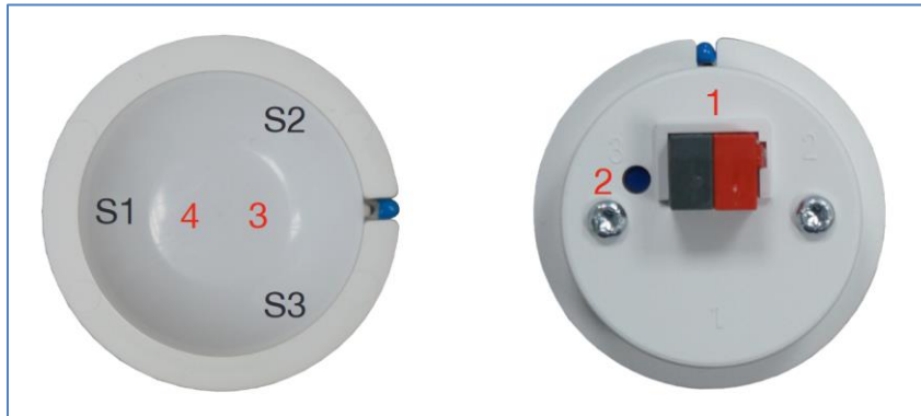
Figure 4: Structure and location of the sensors/LEDs – SCN-P360E3.03
