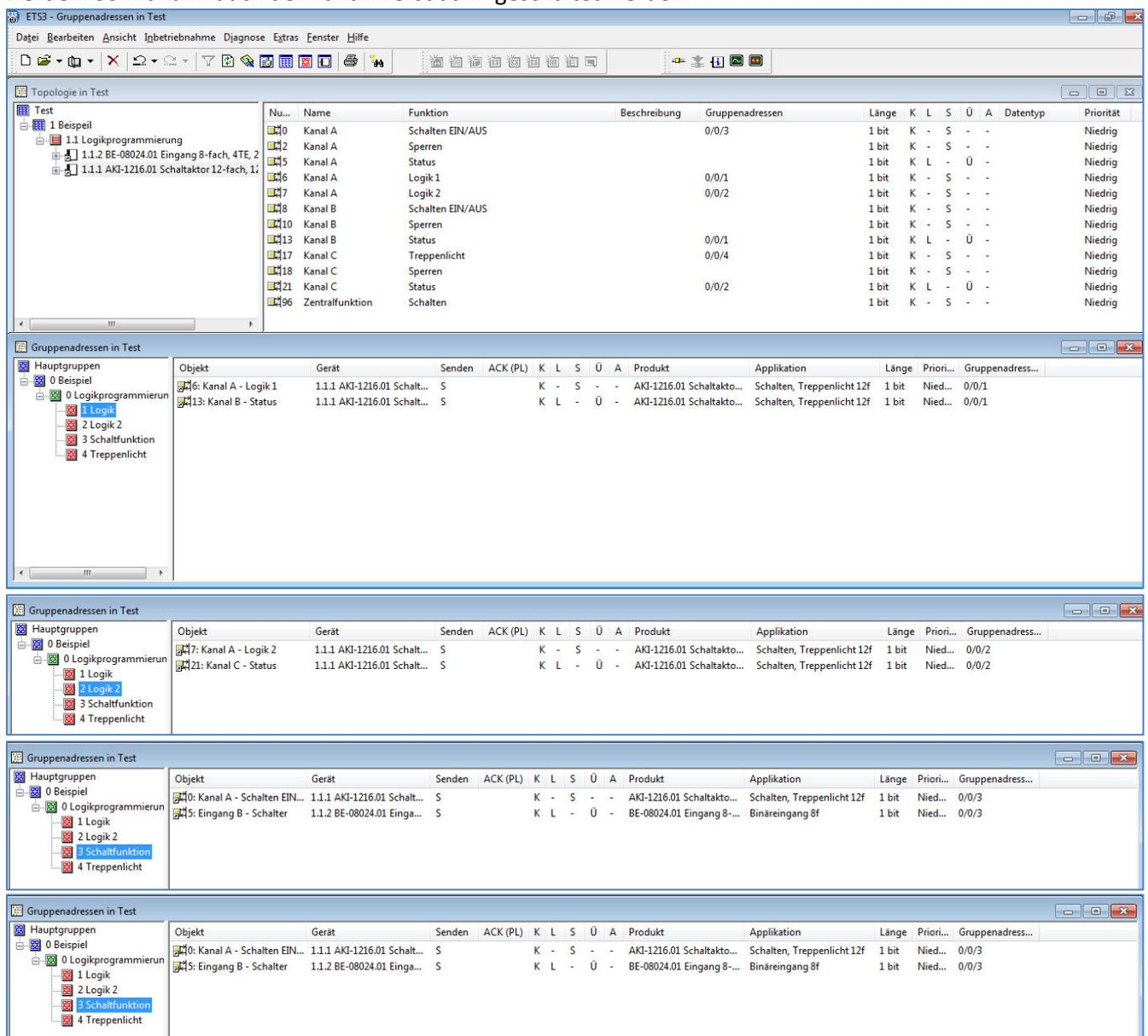
The screenshot displays the ETS3 software interface for configuring logic programming. It shows a hierarchical tree on the left and a main table of objects. The 'Gruppenadressen in Test' table is shown in four different states, illustrating the configuration of logic gates (AND, OR) and their associated group addresses.
